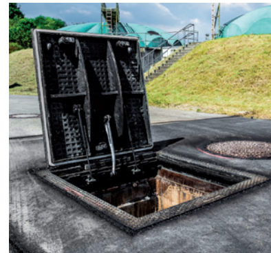
Surface-water-tight cast-iron cover with an opening aid, a load class of D400 and a clear opening of 1000 mm x 1000 mm – Munich
