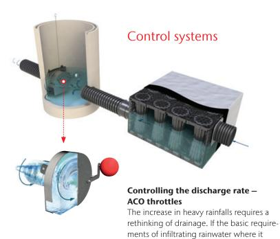
Throttles as the ACO Q-Brake vortex throttle system may be used to flow control the release of the water from the storage into the watercourse. This helps to replenish groundwater levels and reduces the load on the sewage system.
